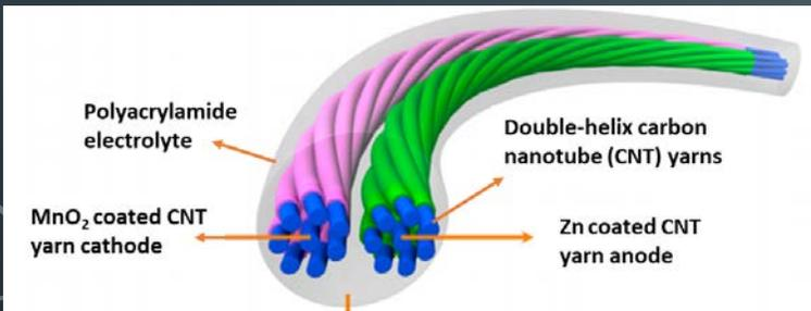
Zinc-Ion class of batteries show good promise. Carbon nano tube yarns coated with MnO<sub>2</sub> and Zn form the anode and cathode of this rechargeable battery yarn.
