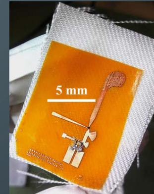
Textile antenna and rectifier (rectenna) enable RF energy to be captured. Large textile surface area is a positive (DOI: 10.1109/WPTC45513.2019.9055541)
