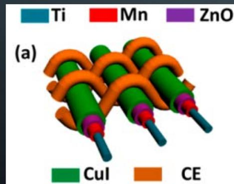
Zinc oxide based dye sensitised solar cell yarns woven with copper coated polymer yarn current collector.
