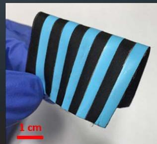
Alternating strips of nylon and PVC form a textile TENG. Works by sliding over a textile electrode.
