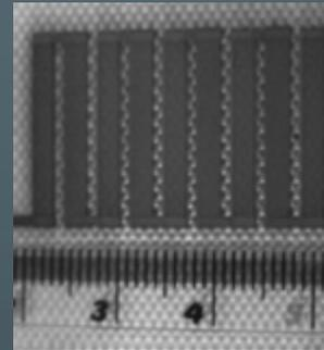
Screen printed SbTe p-type and BiTe n-type thermoelectric module on glass fibre textile.
