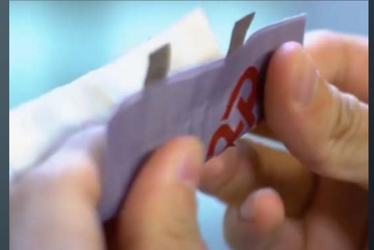
A Textile Lithium Battery uses Cu and Ni coated metallic fabrics as current collectors. Active materials are added to form the cathode and anode and the metallic fabrics, together with separator and electrolyte, are assembled into the battery. DOI: [10.1038/s41467-018-06879-7](https://doi.org/10.1038/s41467-018-06879-7)
