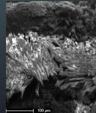
Supercapacitors can be formed in a single textile by controlling the depth of the electrodes
